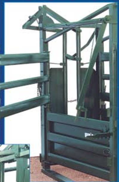
Above: Rear control arm, split opening gates & squeeze.
