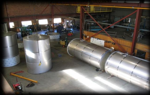
Fully equipped Stainless Steel Fabrication workshop with overhead crane, automatic welding facilities, pulse welding, tank knuckling, coil handling, full MIG and TIG welding
